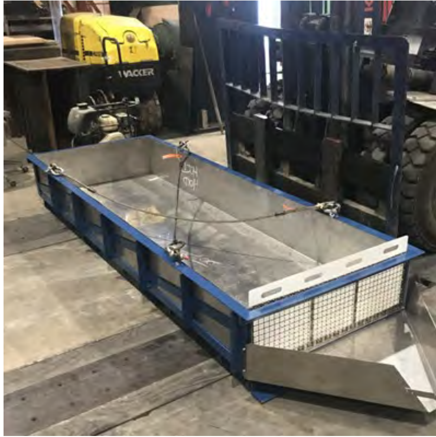
Figure 4.1 Roadbed test frame. 3-feet wide, 9-feet long, stainless-steel lined. Crossed cables used to assist with lifting frame onto steel I-beams. Plastic endpiece removed after roadbed was compacted into test frame. Stainless-steel discharge chute conveyed runoff into flow-through sample bucket.
