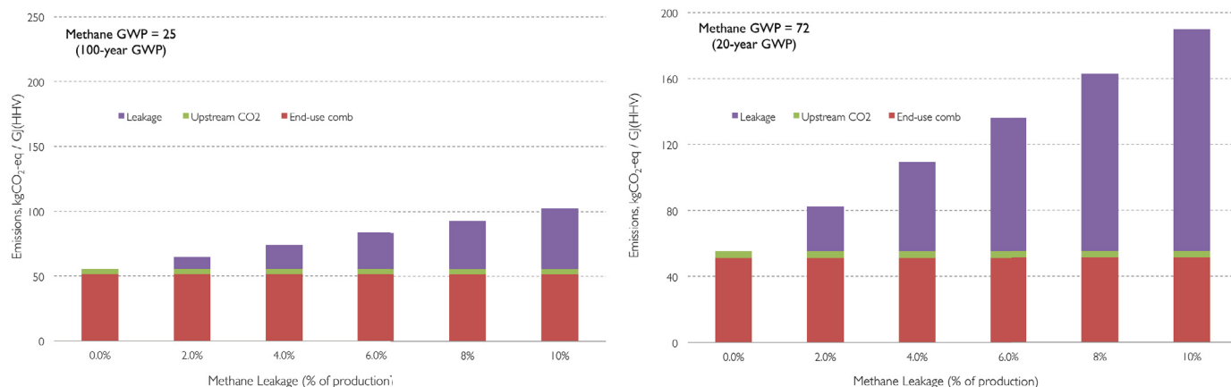
Figure 20. Estimates of greenhouse gas emissions from natural gas production, processing, delivery, and end-use for different assumed rates of upstream methane leakage.
