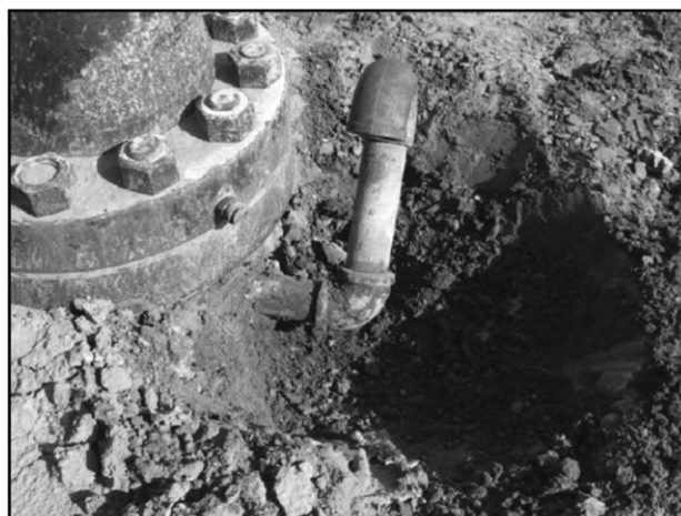
Fig. 2—Diagram and photograph of typical wellhead with surface-casing vent installed (BP: blowout preventer).
